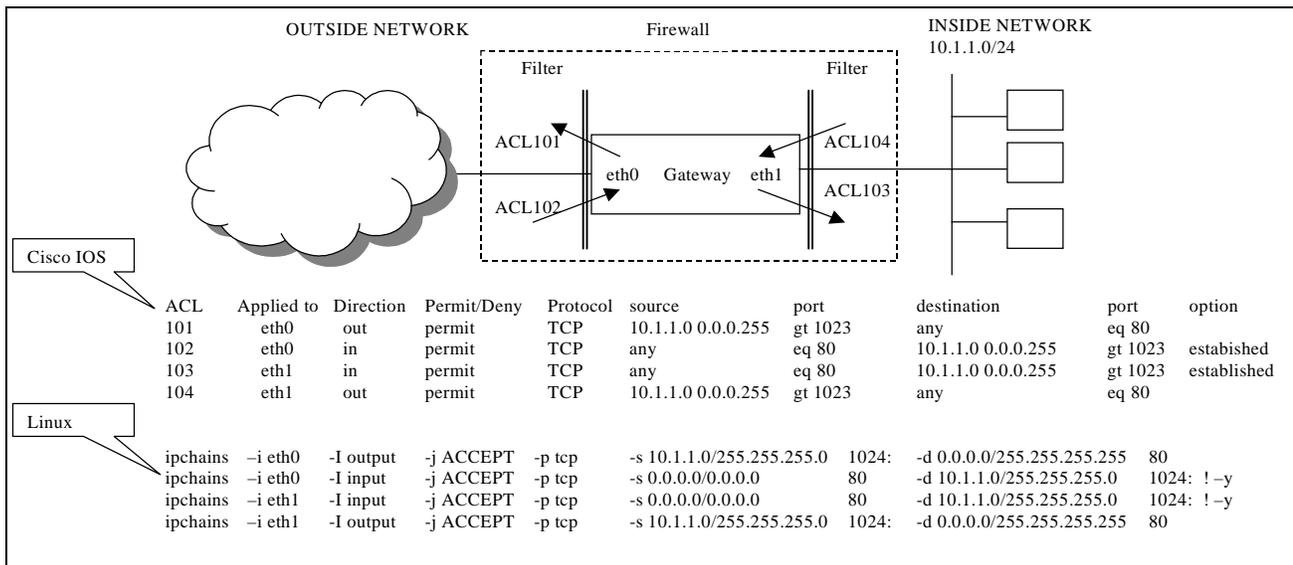
**Figure 15. Cisco IOS Access Control Lists and Linux ipchains**
