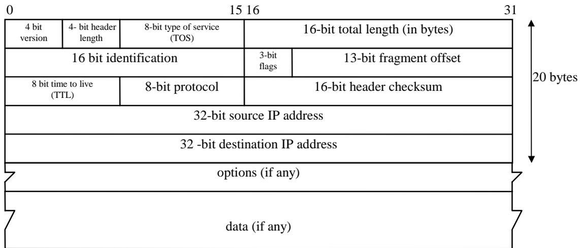
**Figure 5. The IPv4 header**
