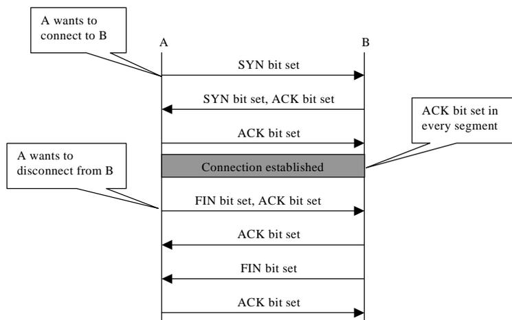
**Figure 14. Setup and tear down of a TCP connection**
