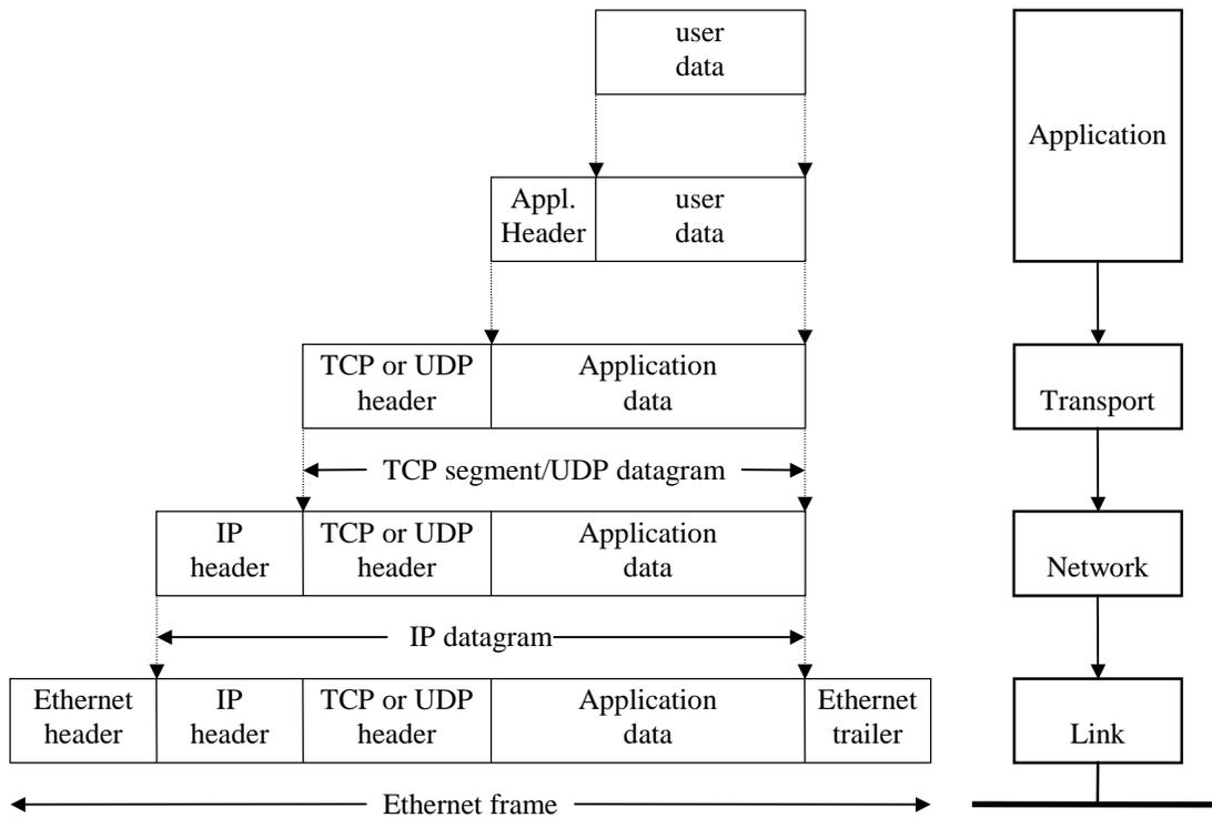
**Figure 2. Encapsulation and layer distribution**
