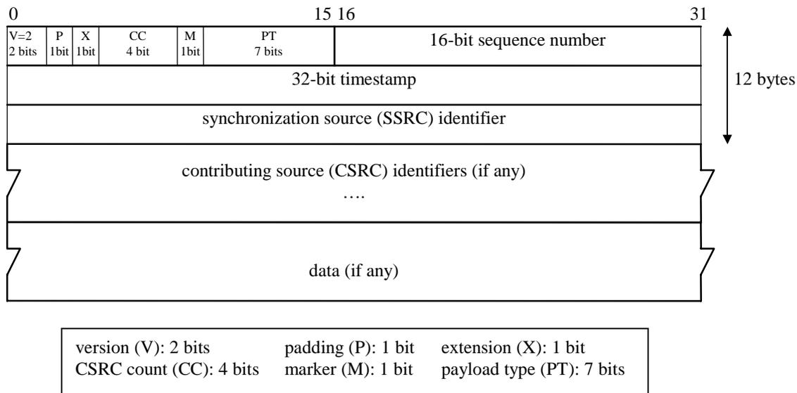
**Figure 1. The RTP header**
