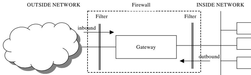
**Figure 13. The principles of a firewall**
